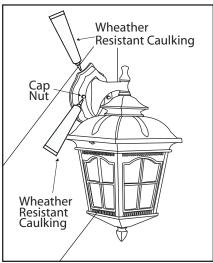
After Installation, seal around the top and side perimeter between the fixture and the wall surface with weather resistant caulking. The bottom should be left un-caulked to prevent moisture build-up. Apply a small amount of weather resistant caulking around the side perimeter between the cap nut and mounting plate.
